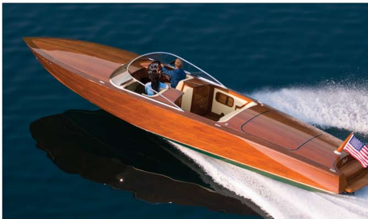
Equipped with twin 400 hp MerCruiser engines, Jefe comes onto plane at just 10 mph, which significantly reduces fuel consumption.
